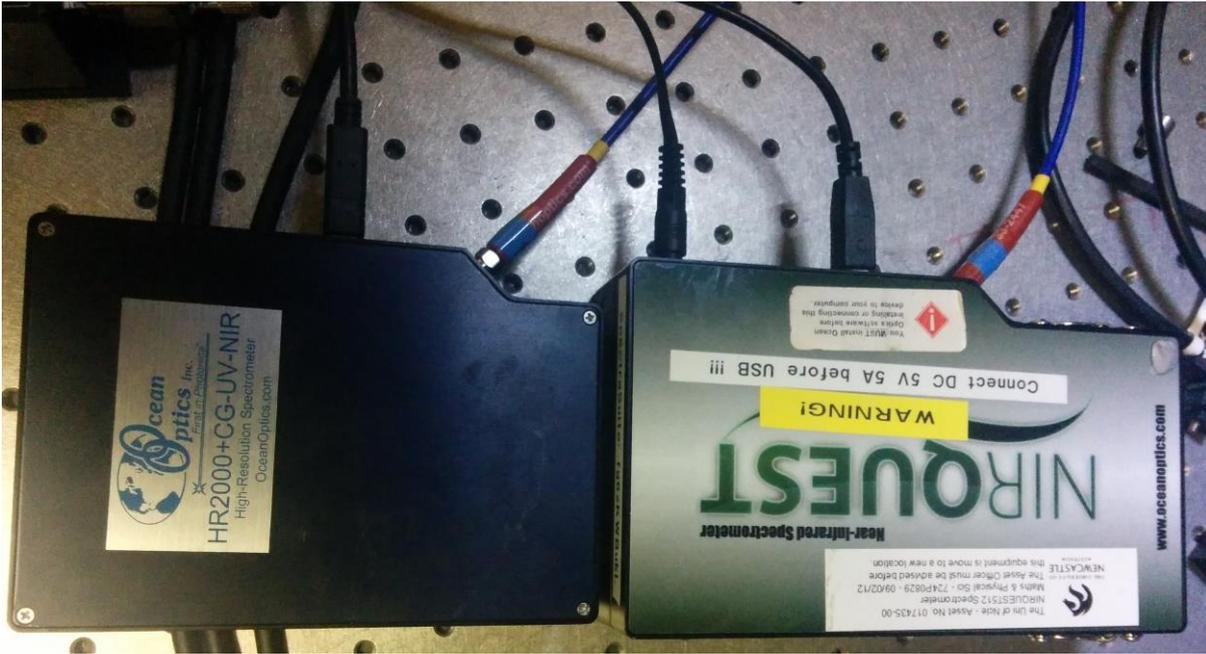
**Figure 2.22: HR2000+ and NIRQuest Spectrometers connected to bifurcated sampling fibre for spectral mode field scanning measurements detailed in section 2.3.5.**
