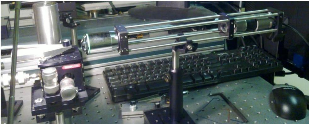
**Figure 2.5: Photograph of fibre microscope capable of resolving some of the MOF structure.**
