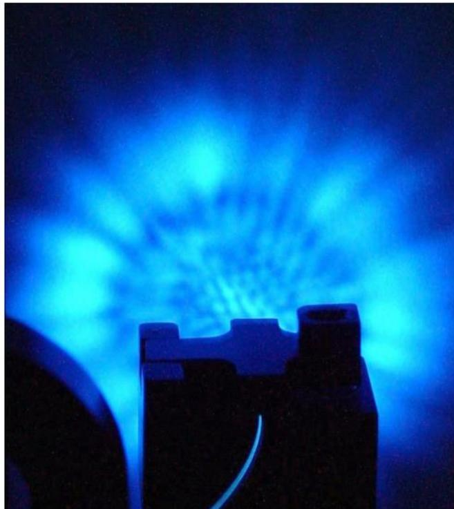
**Figure 1.27: Far field image of MOF supercontinuum generated UV light, clearly in a high order mode [28].**
